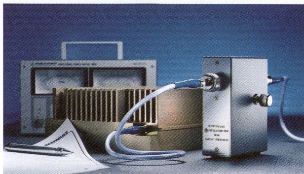
FIG 3 Power measurement at output of 1.8-GHz amplifier using NAS-Z7
