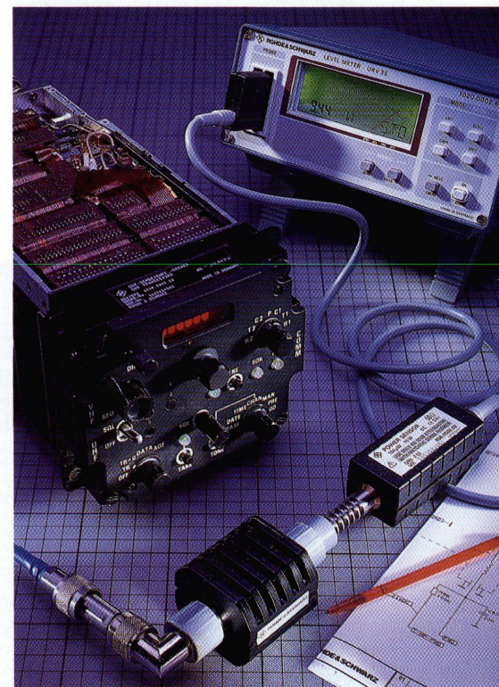
Checking output power of UHF transceiver using Power Sensor NRV-Z53 and Level Meter URV 35 Photo 50 057
