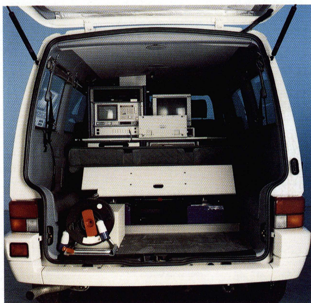
FIG 1 Impulse Response Analyzer PCS is an important tool in planning DAB networks thanks to its wide dynamic range, capabilities for analyzing long delays and measuring raw bit error rates, automatic noise suppression and interfering-signal analysis. Photo 41 564/5
